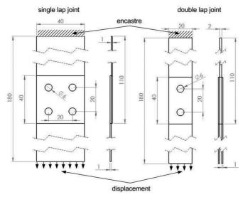
Fig. 2. Types of analysed joints
