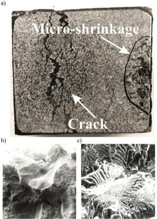
Fig. 1. Non-alloyed cast steel; a) oxidized surface of hot cracks and the shrinkage porosity, magn. 3×; b) the type II sulphides revealed at the surfaces of the intergranular fracture, magn. 250×; c) the type II sulphides, magn. 600×
