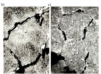
Fig. 2. Shrinkage macro- and micropores in the cracked mill roll of L180HMF cast steel; a) cracks along the boundaries of solidification grains, magn. 5×; b) cracks in the secondary cementite net, magn. 100×; c) cracks in the ledeburite net, magn. 60×; etched with Nital
