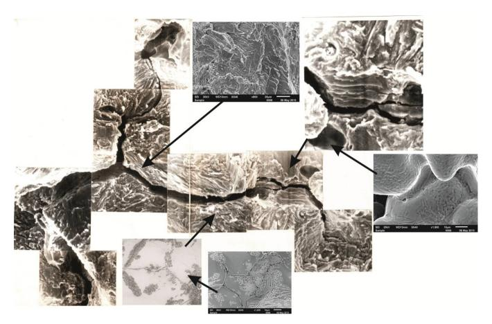
Fig. 4. Hot crack initiated by shrinkage spreading on the bondaries of large grains of solidification and details of eutectics. Scanning microscope
