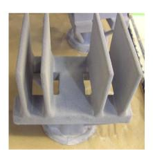
Fig. 2. a) Wax model set b) ceramic mold - after first layer application
