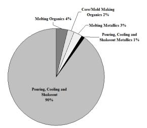
Fig. 1. Participation of individual operations of the process of castings made in moulding sands with bentonite and lustrous carbon carriers - in the emission of contaminations [2]
