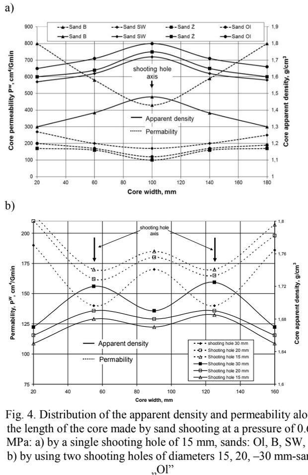
Fig. 4. Distribution of the apparent density and permeability along the length of the core made by sand shooting at a pressure of 0.65 MPa: a) by a single shooting hole of 15 mm, sands: OI, B, SW, Z, b) by using two shooting holes of diameters 15, 20, –30 mm-sand „OI”
