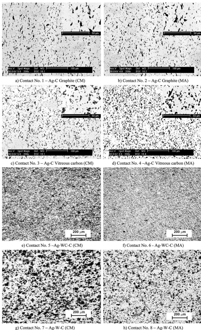
Fig. 3. Microstructures of the tested contact tips
