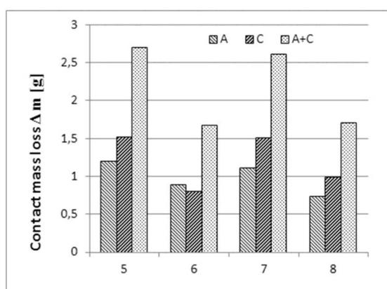
Fig. 6. Results of arc erosion tests at 6 kA current ( $f_{idt}=34$  As),  $N=10$ : 5 – Ag70-WC29.5-C0.5 (CM), 6 – Ag70-WC29.5-C0.5 (MA), 7 – Ag70-W29.5-C0.5 (CM), 8 – Ag70-W29.5-C0.5 (MA)
