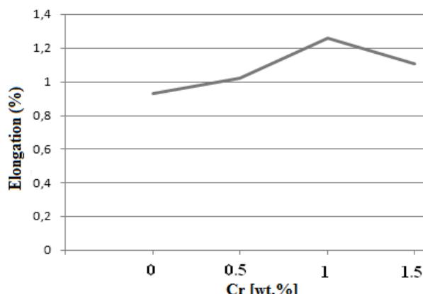
Fig. 8. Ductility of alloys after chrome addition
