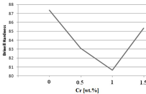
Fig. 9. Brinell Hardness of alloys after chrome addition
