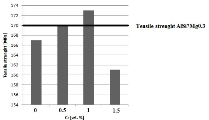
Fig. 6. Tensile strength of alloys after chrome addition
