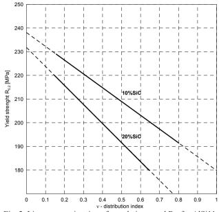
Fig. 2. Linear approximation of correlation v and R<sub>02</sub> for AlSi11-10%SiC i AlSi11-20%SiC composites.
