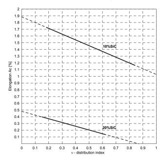
Fig. 3. Linear approximation of correlation vand A<sub>5</sub> for AlSi11-10%SiC i AlSi11-20%SiC composites.
