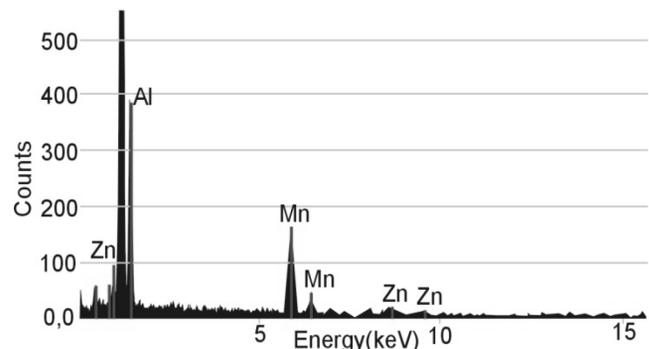
Fig. 9. Local chemical analysis of the precipitates containing Mg, Al, Mn and Zn in sample 2
