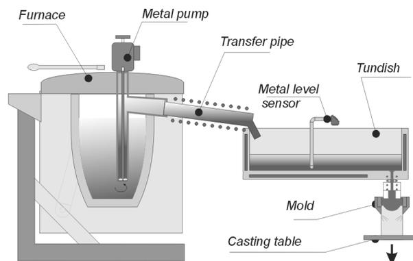
Fig. 1. A diagram of the VDC installation for casting of billets in magnesium alloys
