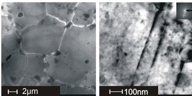
Fig. 7. The microstructure of sample 2 equiaxed grains and slip bands
