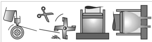
Fig. 3. Schematic representation of the cast material fabrication process by Rapid Solidification
