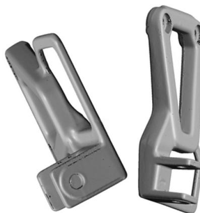
Fig. 5. Unscanned places of the part (black color)
