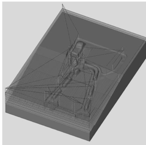
Fig. 7. Simulation of roughing cycle - the bottom part of the mold cavity
