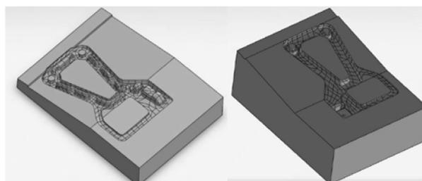
Fig. 6. Virtual design of mold cavity
