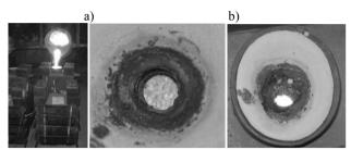
Fig. 3. Pouring trials, a) mold with filter, b) damaged filter
