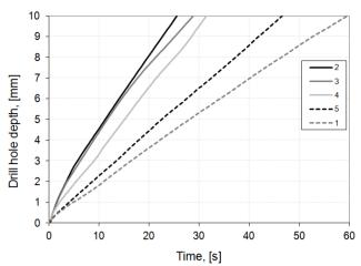
Fig. 2. Cutting curves of the investigated alloys
