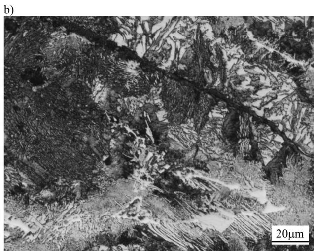
Fig. 4 (a, b). The microstructure of grey cast iron in cellulose profile: flake graphite, pearlite, ausferrite, carbides
