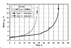
Fig. 2. Creep characteristics of nickel superalloy IN-713C under the conditions of the I variant
