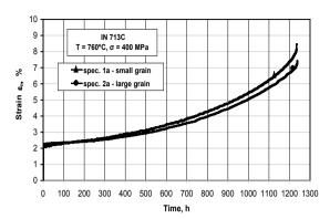
Fig. 4. Creep characteristics of IN-713C nickel superalloy under the conditions of the II variant
