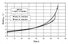
Fig. 5. Creep characteristics of MAR-247 superalloy under the conditions of the II variant
