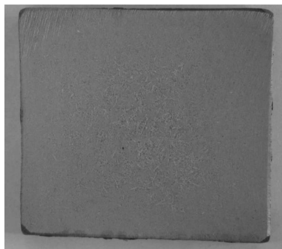
Fig. 4. Macrostructure of pig (etching 20% NaOH)
