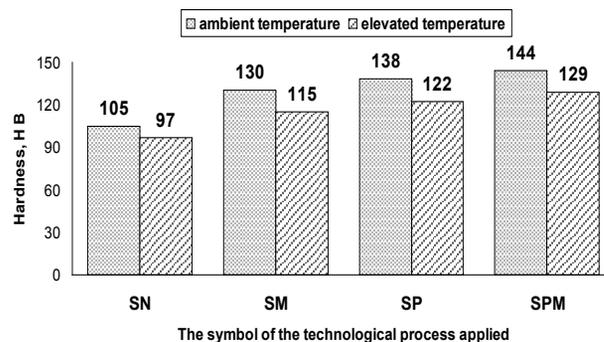
Fig. 1. The result of HB hardness testing results for technologies
