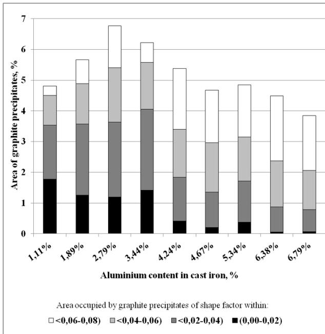
Fig. 7. The influence of aluminium content in cast iron on the area occupied by graphite precipitates
