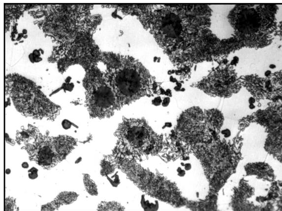
Fig. 6. Microstructure of cast iron containing 6.79% Al; etched with Nital, magn. 300×
