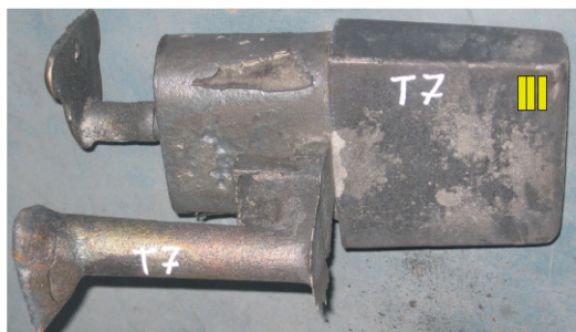
Fig. 1. Sample casting after knocking-out with marked position of specimens for abrasive tests
