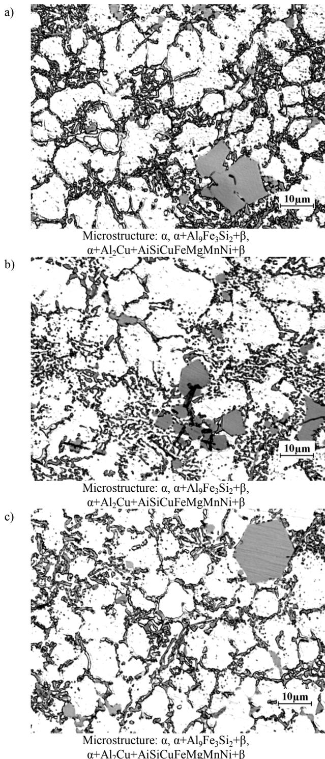
Fig. 2 (a-c). Representative microstructures of 226 silumin pressure casts: non-modified (a), after Sr modification (b) and after Sb modification (c)
