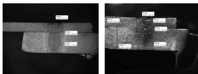
Fig. 3. Good quality of laser weld, 80% of penetration
