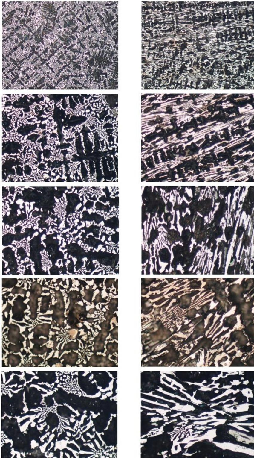
Fig. 12. Microstructure on perpendicular (left) and parallel (right) sections to the direction of heat removal distant from the model mould of 5, 20, 40, 60, 85 [mm], mag. 200x, etched
