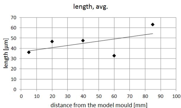
Fig. 9. The average length of carbides on parallel sections
