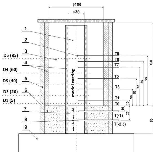
Fig. 1. Construction of the ATD-Is100 tester with indicated position of thermocouples and specimens used in the analysis, 1 – model casting, 2 – S-type thermocouple, 3 – thermal insulator, 4 – insulating material Sibral 300, 5 – steel casing, 6 – moulding material (quartz sand), 7 – model mould, 8 – K-type thermocouple, 9 – base, T0 – S-type thermocouple located on the border of the model casting – model mould, T1 ÷ T9 – S-type thermocouples placed in the model casting [2]
