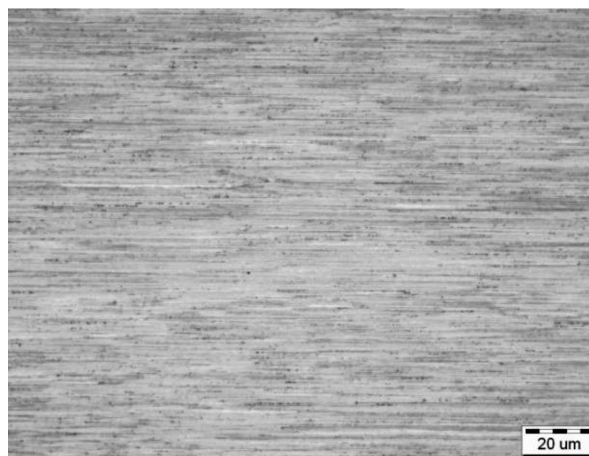
Fig. 7. Microstructure of Cu-Ag wire of diameter 0,50 mm, longitudinal section
