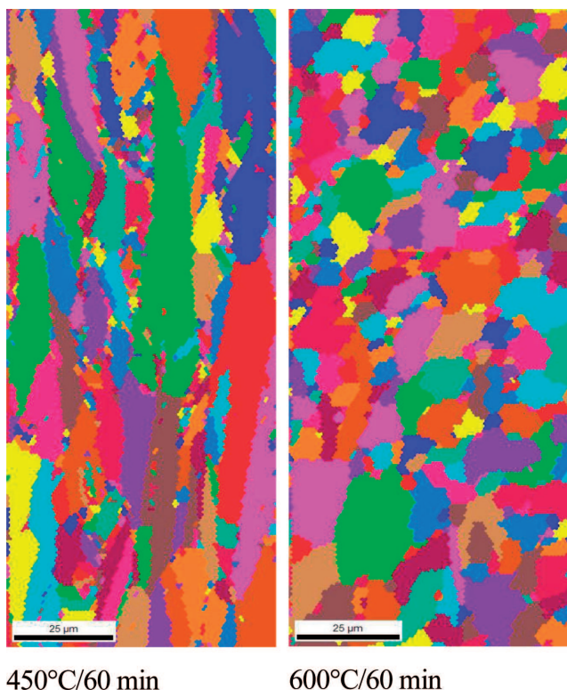
Fig. 4. Maps of grain size in CuFe 2 alloy – quenched, cold deformed with 50% reduction and aged in temperature of 450°C for 60 and in temperature 600°C for 60 minutes
