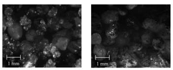
Fig. 2. Sandmix with phenol-formaldehyde resin before (left) and after utilization (right)
