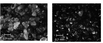
Fig. 1. Sandmix with phenolic resin before (left) and after utilization (right)
