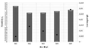
Fig. 3. Permittivity and loss factor for waste moulding and core sands
