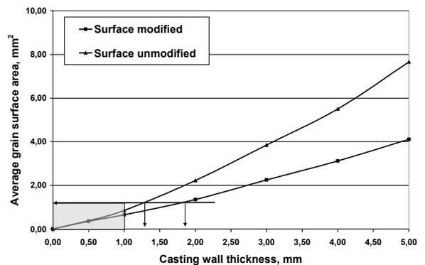
Fig. 9. Average grain surface area as a function of casting wall thickness for modified and unmodified sides
