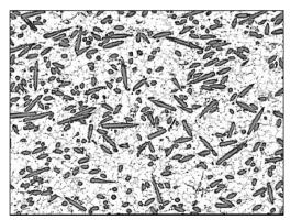
Fig. 2. Microstructure of the AlSi9Mg/10% CF composite, magn. 100×
