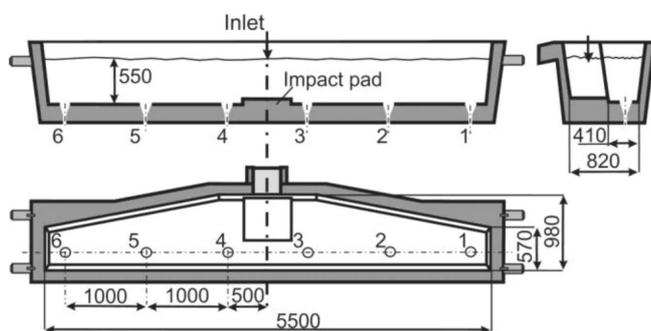
Fig. 1. Geometry of the studied industrial tundish, dimensions in [mm]
