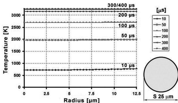
Fig. 7. The temperature distribution along the radius of nickel powder with a diameter of 25  $\mu\text{m}$  after 10, 50, 100, 200, 300 and 400  $\mu\text{s}$
