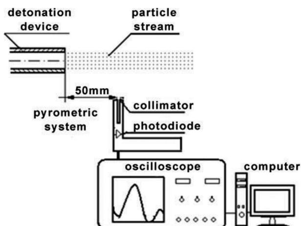
Fig. 2. System for measuring the stream temperature [7]
