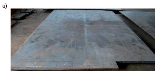
Fig. 2. Example strain history (for single strain gauge) registered in titanium during the drilling process, (a) – the specimen cut out just after explosive welding process, (b) – the specimen after the heat treatment and cold rolling
