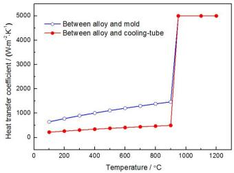
Fig. 4. Relationship between heat transfer coefficient and temperature
