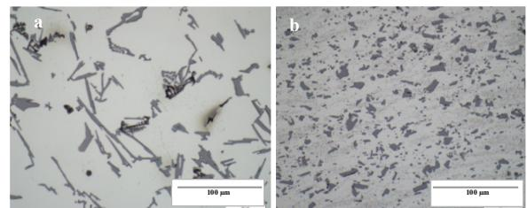
Fig. 18. Structures of casting alloy before FSW – a) and after FSW process – b) (SEM)
