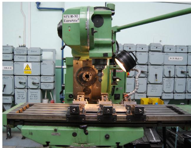
Fig. 2. Station for FSW welding process testing
