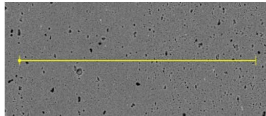
Fig. 14. Fragment of the structure from Fig. 8. Welding parameters:  $\omega = 900 \text{ min}^{-1}$ ,  $V = 224 \text{ mm/min}$ . Triflute pin. SEM-EDS chemical composition analysis was conducted along the marked line (Fig. 15)
