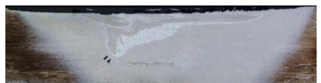
Fig. 8. Structure of FSW weld in the case of locating the rod of EN AC-43200 (A) on the advancing side. Welding parameters:  $\omega = 900 \text{ min}^{-1}$ ,  $V = 224 \text{ mm/min}$ . Triflute pin. Etching: Keller
