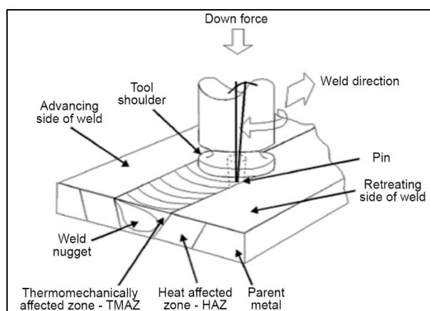
Fig. 1. The scheme of the FSW process [1]
