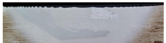
Fig. 7. Structure of FSW weld in the case of locating the rod of EN AC-43200 (A) on the retreating side. Welding parameters:  $\omega = 450 \text{ min}^{-1}$ ,  $V = 224 \text{ mm/min}$ . Triflute pin. Etching: Keller
