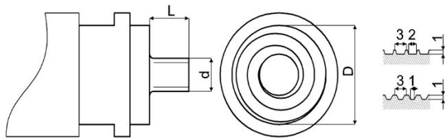
Fig. 3. Structure of a working part of FSW process tool
