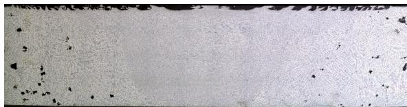
Fig. 16. Macrostructure of FSW weld (in the central zone) in the EN AC-43200
