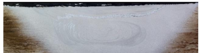
Fig. 9. Structure of FSW weld in the case of locating the rod of EN AC-43200 (A) on the retreating side. Welding parameters:  $\omega = 900 \text{ min}^{-1}$ ,  $V = 224 \text{ mm/min}$ . Triflute pin. Etching: Keller
