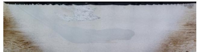
Fig. 6. Structure of FSW weld in the case of locating the rod of EN AC-43200 (A) on the advancing side. Welding parameters:  $\omega = 450 \text{ min}^{-1}$ ,  $V = 224 \text{ mm/min}$ . Triflute pin. Etching: Keller
