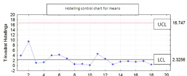
Fig. 4. Hotelling control chart for means (source: Stat-Soft).
