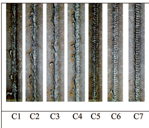
Fig. 6. Vibration-laser interfusions made using Sample No. 3
