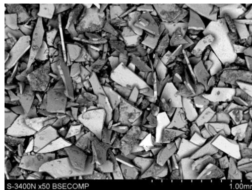
Fig. 1. Morphology of Nd_{11}Fe_{77}Co_5B_6 powder after encapsulation with Ni-P
