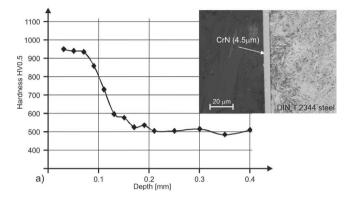
Fig. 3. The results of metallographic investigations and the changes of hardness in nitrided layers developed for the tested layered composites
