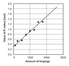
Fig. 7. Results of the measurement of the R radius value changes in the function of a number of steel synchronizer rings forgings produced for dies coated with "nitrided layer / CrN coating" layered composites
