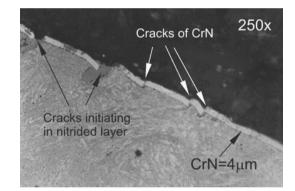
c) CrN (4 µm)/2000 forgings
