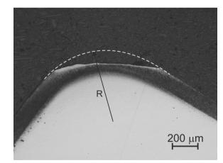
Fig. 8. The results of metallographic investigations for the die coated with a "nitrided layer/ CrN coating" layered composite after forging 2000 of steel synchronizer rings
