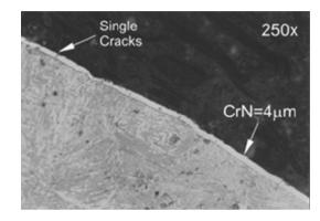
b) CrN (4 µm)/1000 forgings
