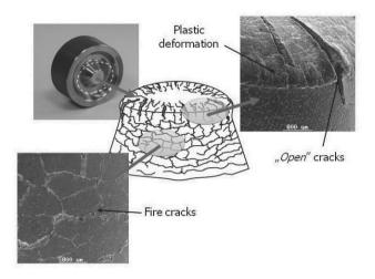
Fig. 5. The main destruction mechanism of destruction of forging dies having the hybrid layer "nitrided layer / CrN coating"
