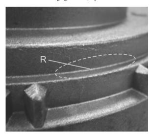
Fig. 6. Steel synchronizer rings forging with marked R radius, whose value determines the durability of the die
