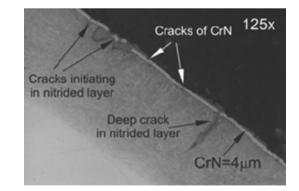
Fig. 4. The analysis of the failure intensity of forging dies with nitrided layer / CrN coating composite layers after their various maintenance time
