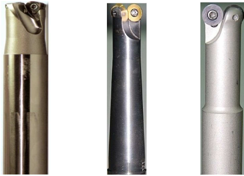
1) Milling cutter AJX06R162SA16S 2) Milling cutter R300-016A20L-08L 3) Milling cutter R390 E45 D16-W25
