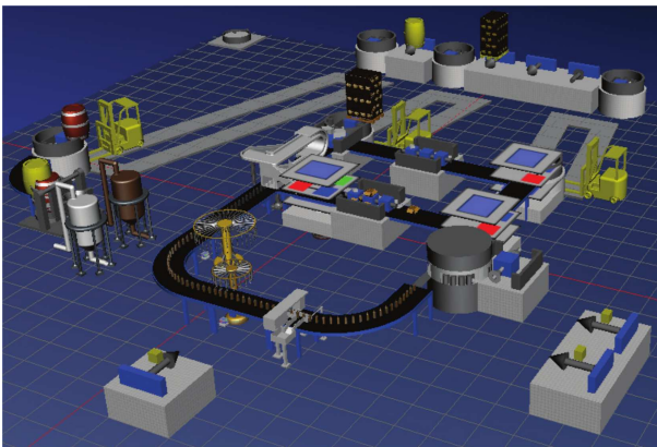
Fig. 8. 3D simulation of beverage technological process in Tecnomatix Plant Simulation.
