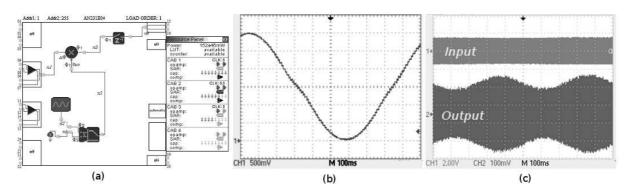
Fig. 5. Tremolo effect application. a) Schematic of the tremolo effect; b) Distorted 1 Hz sinewave generated by the LFO; c) Input and output signals of the tremolo
