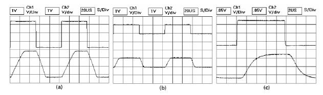
Fig. 1. Pulse response for large (a), small (b) and very small (c) amplitude
