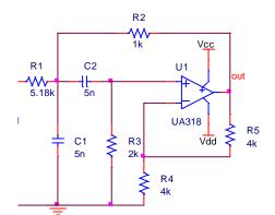
Fig. 3. Sallen-Key band pass filter.
