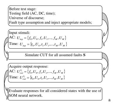
Fig. 1. Testing procedure.
