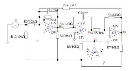
Fig. 5. An analog filter.
