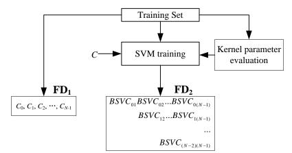
Fig. 2. Construction of two fault dictionaries.
