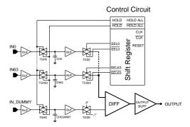
Fig. 6. Simplified scheme of the multiplexer.
