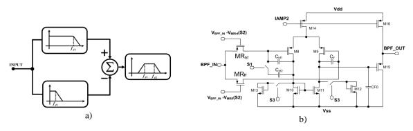
Fig. 5. Band pass filter: a) simplified block diagram, b) simplified scheme of the filter.
