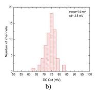
Fig. 8. Spread of analog parameters in 64-channel ASIC: (a) gain, (b) output offset.
