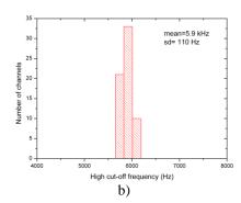
Fig. 9. Spread of analog parameters in 64-channel ASIC: (a) low cut-off frequency, (b) high cut-off frequency.
