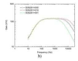
Fig. 7. Measured frequency response of a single channel for: a) tuning the time constant of the input AC-coupled circuit, b) different values of switches S1, S2, S3 to change the high cut-off frequency.
