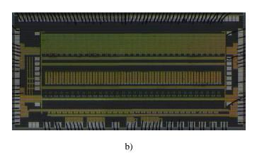
Fig. 1. Multichannel recording ASIC: a) block diagram, b) photo of a 64-channel chip: input pads are at the top side, control and output pads are at the bottom side, power supply and test pads are on the left and right side.
