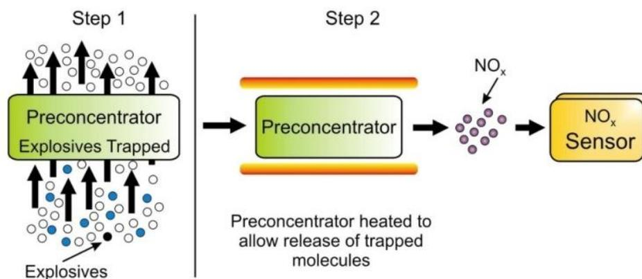
Fig. 12. Idea of the concentration and thermal decomposition of explosives vapour.
