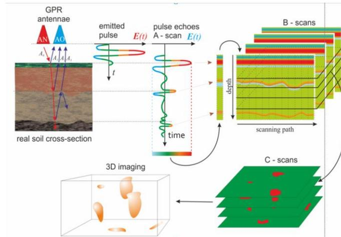
Fig. 8. Different kind of GPR imaging formation.
