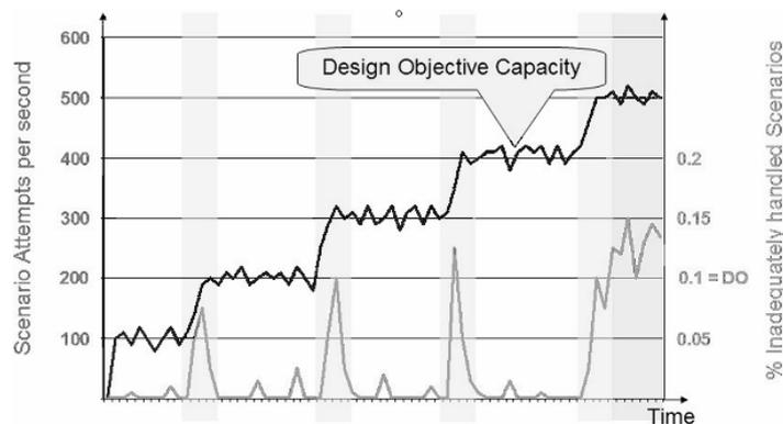
Fig. 2. Typical ETSI performance test sequence [9].
