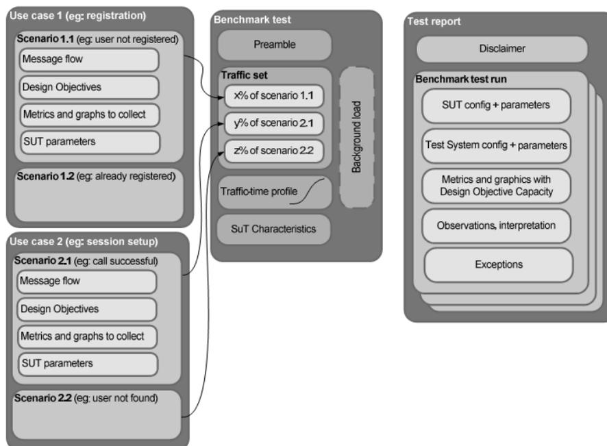
Fig. 1. ETSI performance measurements information model [6].
