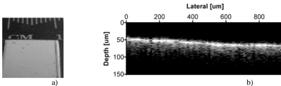
Fig. 8. Sample with anti-corrosion coating; a) sample image, b) OCT cross-sectional image.
