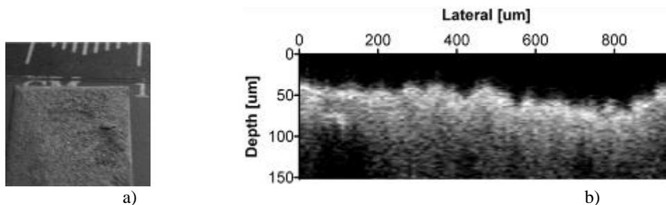
Fig. 10. Corrosive sample destruction; a) sample image, b) OCT cross-sectional image.
