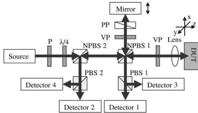
Fig. 1. The PS-OCT setup; PBS 1÷2 – polarization beamsplitter, NPBS 1÷2 – non-polarization beamsplitter, PP – dispersion compensation prism, P – polarization plate,  $\lambda/4$  – quarter-wave plate, VP – variable wave plate; DUT – device under test.
