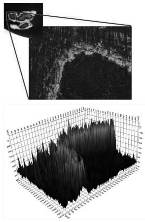
Fig. 4. The image of the Ti-1Al-1Mn alloy surface after 6 hours of oxidation (a), the surface topography of the selected area (b)
