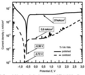
Fig. 6. Potentiokinetic polarization curves of Ti-1Al-Mn alloy. Experimental conditions: artificial saliva solution, potential scan rate 10 mV s<sup>-1</sup>, temperature  $37^{\circ}C$
