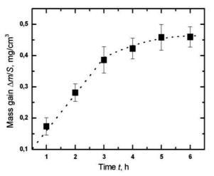
Fig. 2. The Ti-1Al-1Mn alloy oxidation kinetic curve (oxidation temperature 800°C)
