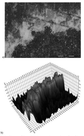
Fig. 5. The image of the Ti-1Al-1Mn alloy surface after 6 hours of oxidation (a), the surface topography (b)
