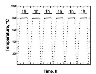
Fig. 1. Scheme of cyclic thermal oxidation of Ti-1Al-1Mn alloy
