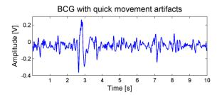
Fig. 2. Ballistocardiograms contaminated with noise due to subject movement, obtained with a 400 x 300 mm<sup>2</sup> film sensor. Slow baseline oscillations (left) and short but strong movements (right).
