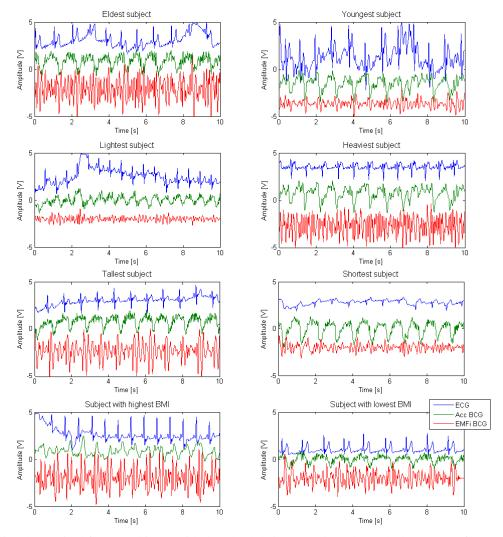
Fig. 7. Signals acquired from 8 subjects, with the wheelchair stopped. Each graph shows ECG from Medlab P-OX100 (blue, upper position within graph) and seat BCG from zz axis of the accelerometer (green, middle position) and EMFi (red, bottom position). The eldest subject is 48 years old, the youngest 18. The lightest has 55 kg, the heaviest 90 kg. The tallest has 1.88 m, the shortest 1.63 m. The highest BMI is 29.4, the lowest 19.4.
