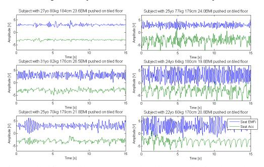
Fig. 8. Signals acquired from 6 subjects, pushed on the wheelchair over the tiled floor shown. The seat EMFi signal (blue upper position) and the seat accelerometer zz axis (green lower position) are shown.
