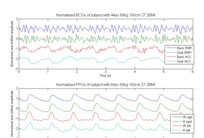
Fig. 5. All the physiological signals gathered by the system implemented in the wheelchair, simultaneously acquired for one of the volunteers. In the top, 4 BCGs, displacement, and acceleration, acquired in backrest and seat. In the bottom, 4 PPGs, red and infrared, acquired in both hands.
