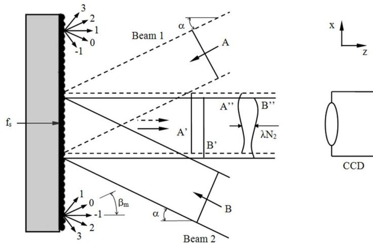
Fig. 1. Moiré interferometry principle [23].
