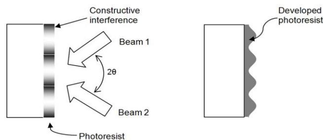
Fig. 2. Holographic grating obtained with photoresist [23].
