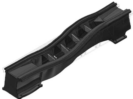
Fig. 11. F4 mode of the iron cast body – frequency 393 Hz
