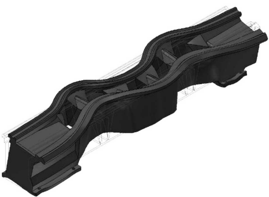
Fig. 14. F8 mode of the iron cast body – frequency 783 Hz
