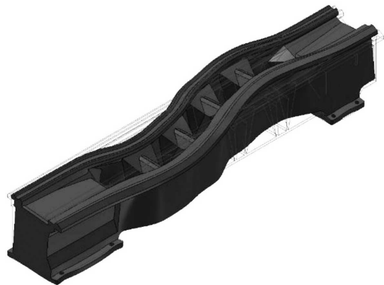
Fig. 12. F4 mode of the hybrid body – frequency 425 Hz
