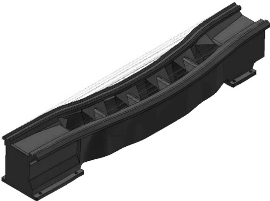
Fig. 10. F1 mode of the hybrid body – frequency 195 Hz
