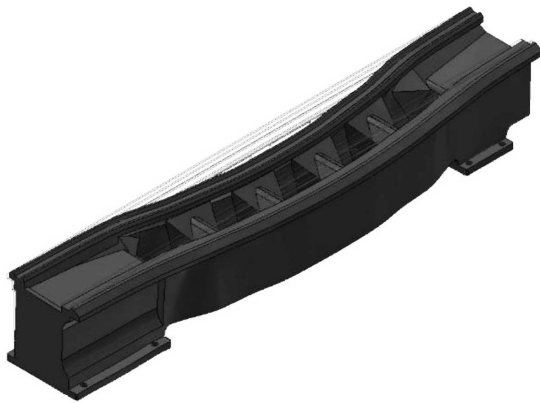
Fig. 9. F1 mode of the iron cast body – frequency 189 Hz
