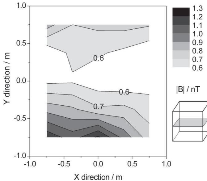
Fig. 6. Magnitude of the residual magnetic field  $|B|$  inside the Zuse-MSR after degaussing, measured at night. Shown is the central X-Y plane of the chamber. The high amplitude at the front right side is caused by the pneumatic buttons for open, close and security ventilation of the door mechanism, which still contains magnetically contaminated components, like springs.
