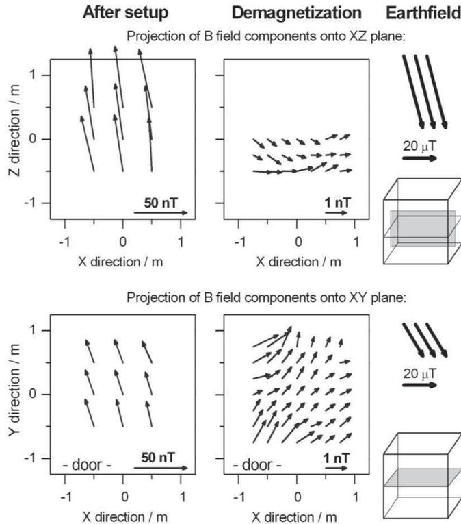
Fig. 5. Magnetic field map inside Zuse-MSR. Above:  $B_x$  and  $B_z$  components shown as projections onto the vertical plane. Below: projection of the  $B_x$  and  $B_y$  components onto a horizontal plane. Left: After installation of the MSR, using a fluxgate. Right: Result after degaussing using a SQUID system. Both measurements were performed at night during the subway break. Root points represent the measurement position. The origin corresponds to the center of the room.
