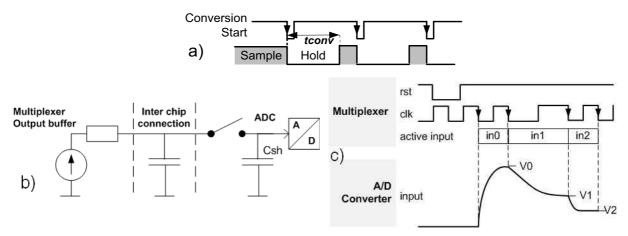
Fig. 11 a) Time diagram of A/D converter Sample & Hold circuit operation, b) Equivalent electric model of multiplexer output to A/D converter signal path, c) Time diagram of A/D converter input voltage switching.
