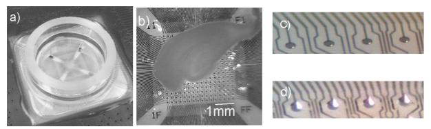
Fig. 5. Multi-electrode array for *in vitro* experiments realised on glass substrate. a) MEA mounted on PCB and surrounded by glass fringe creating a chamber for liquid. b) MEA with hippocampus tissue slice. c) planar electrodes. d) tip shaped electrodes. (Photos taken from the presented system).
