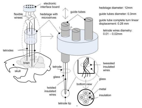
Fig. 2. Scheme of setup for *in vivo* multi-point neural activity recording by using tetrodes. Exemplary dimensions of key elements are taken form [10]. (The author's drawing).
