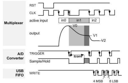
Fig. 12. Diagram of the conversion and transmission of a single voltage sample from a single conditioning channel with respect to time.
