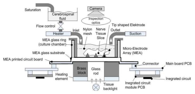
Fig. 13. Sketch of experimental setup for multichannel in vitro multichannel neural activity recording.
