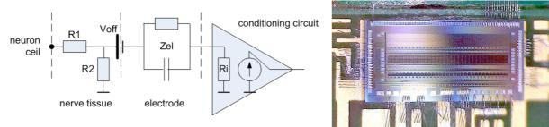
Fig. 7. Circuit model displaying the connection between the neuron and conditioning circuit.
